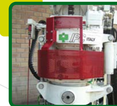
8 MANDRINO JET GROUTING JET GROUTING CHUCK CABEZA PASANTE PARA JET GROUTING
